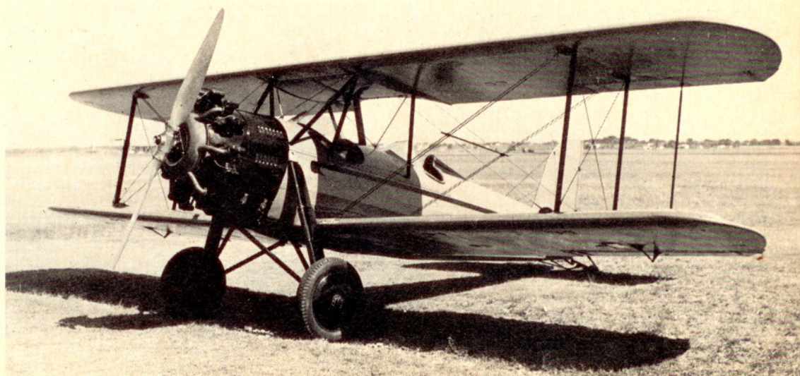
This three quarter front view of the 225-hp C3-225 model shows the straight-across top wing and dihedralled lower wing that were C3 trademarks.
